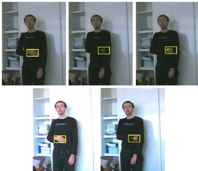
Figure 1: Test sequence for occlusion diagnosis. The reference model is defined in the first image. Partial (images 3 and 5) and total (image 2) occlusions are correctly detected, as indicated by 'P' and 'O' letters, while illumination change (image 4) is not mistaken for occlusion. Here the adaptation process is applied as soon as no partial or total occlusion is detected, and a particle filter is used to track the hand.
