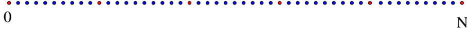
Figure 2: The repatoms (in red) are explicitly treated, all other atoms (in blue) being eliminated in the CG procedure.
