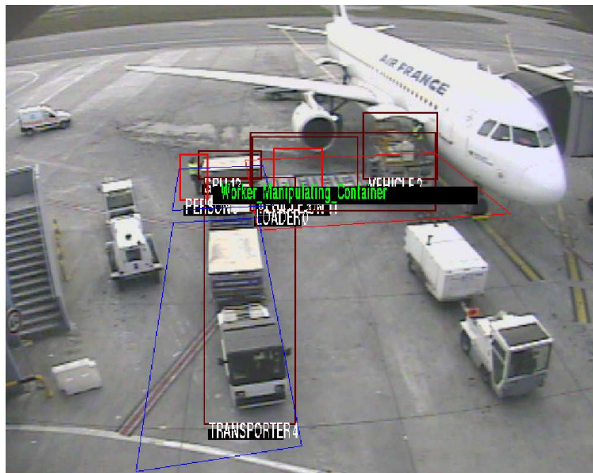
Fig. 5 This Composite state is recognised when the apron worker is manipulating a container in the working zone. This is recognised when the worker has arrived in this zone and that a container is detected in it. This enables to recognise that they are interacting with each others.
