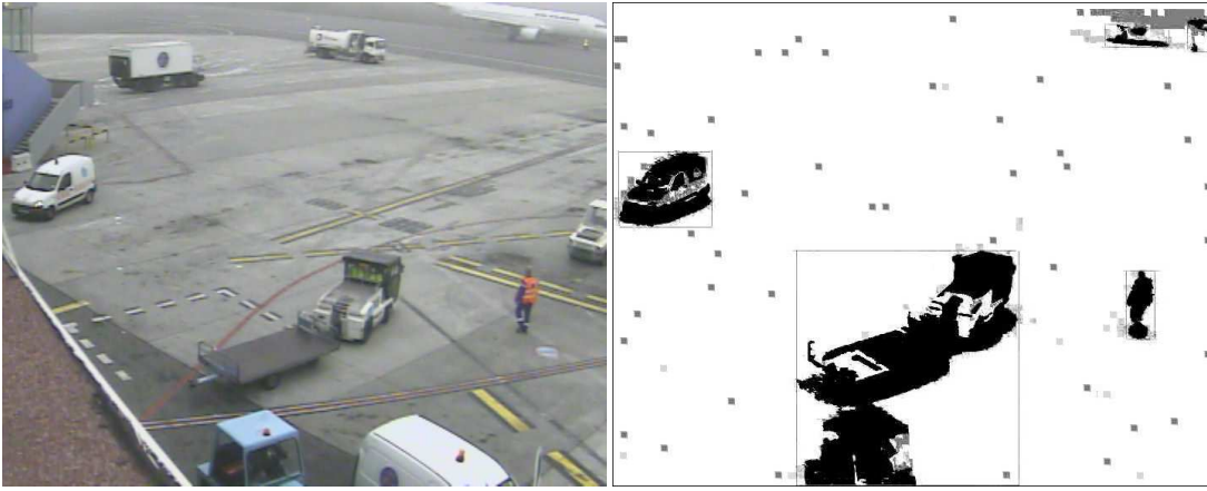
Fig. 6 Representative motion detection result from dataset 1 showing (Left) reference image and (Right) detection result for the colour mean and variance algorithm.
