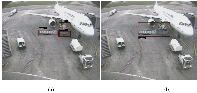
Fig. 3 (a) Before the Global Tracker, a Loader vehicle is detected as several mobile objects (over detection). (b) After the Global Tracker, the Loader vehicle is correctly tracked as one mobile object.
