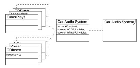
Figure 2: Class diagram for the Car Audio System.
