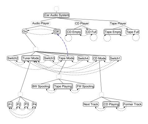
Figure 3: State machine model of the Car Audio System and the associated tree structure.
