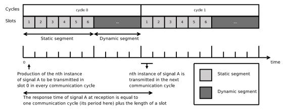
Figure 2: Example showing that the slot location matters even in the case where the signal deadline is equal to its period.
