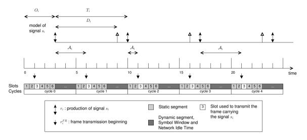
Figure 1: Illustration of the system model. Successive signal instances are produced and transmitted in the third slot of every communication cycle where  $r_i$  is the release time of an instance of the signal  $s_i$  and  $r_i^{FR}$  is the beginning of transmission of an AUTOSAR frame sending  $s_i$ .
