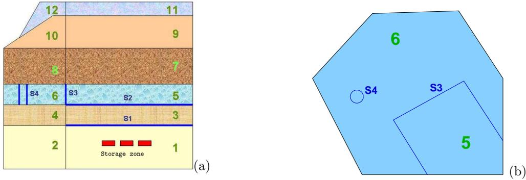
Figure 1: 2D vertical section (a) and horizontal section (b) of the 3D hydraulic model.  $S_1, \dots, S_4$  are the outlet channels. Green numbers are the indices for zones.  $\mathbf{K}_1 = \mathbf{K}_2 = \text{diag}(k_h, k_h, k_v)$ ,  $\mathbf{K}_i = k_i \mathbf{I}$  for  $i = 3, \dots, 12$ .  $k_h, k_v$  and  $k_i, i = 3, \dots, 6$  are uncertain.
