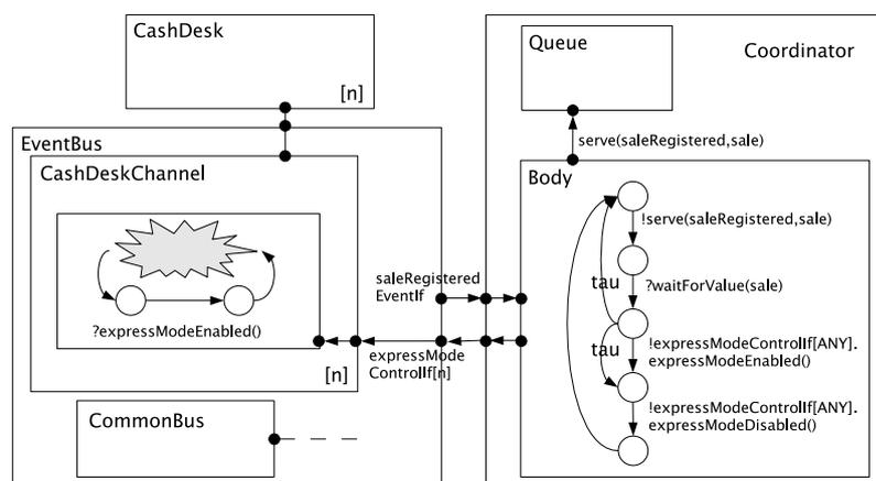
Figure 11: A partial pNets model of CoCoME
