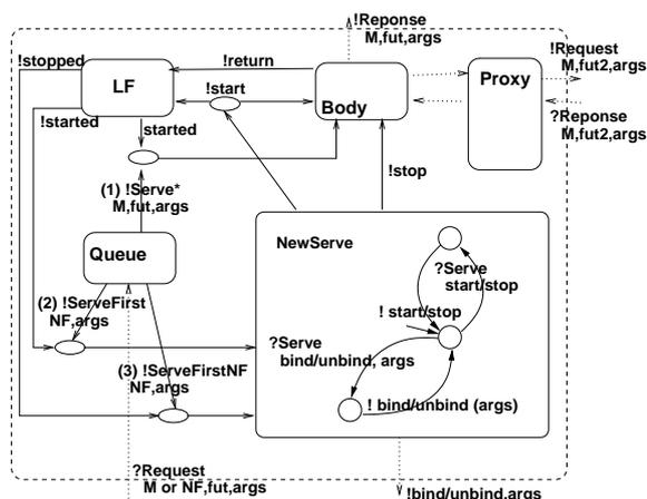
Figure 7: Behaviour model for a GCM/ProActive Primitive
