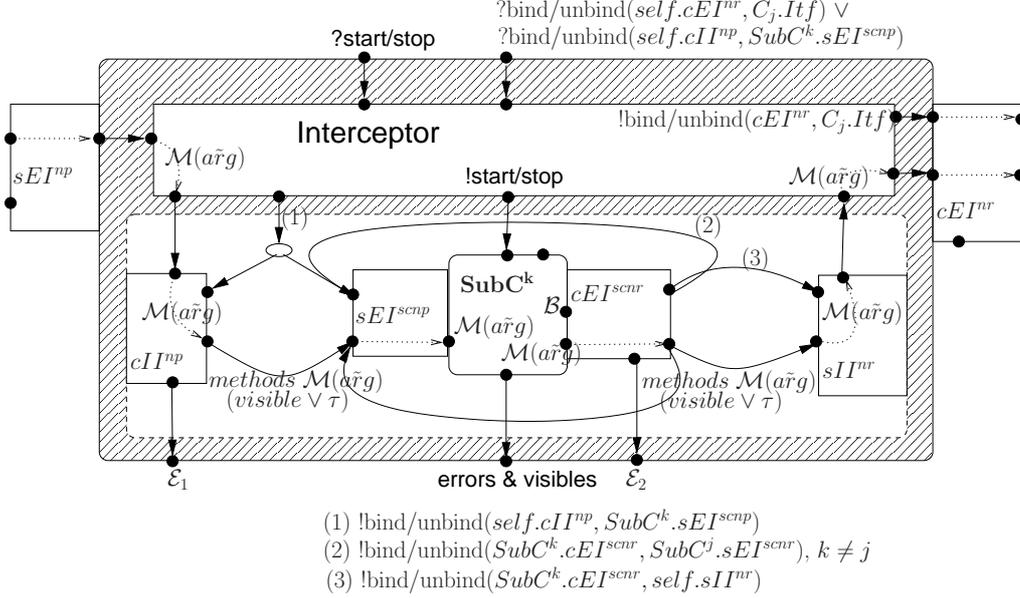
Figure 5: Synchronisation pNet for a Fractal Composite Component
