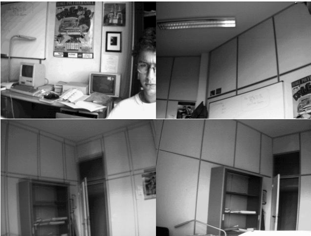
Fig. 4 Some of the images that were used for distortion calibration. Even blurred or fuzzy pictures can be used.
