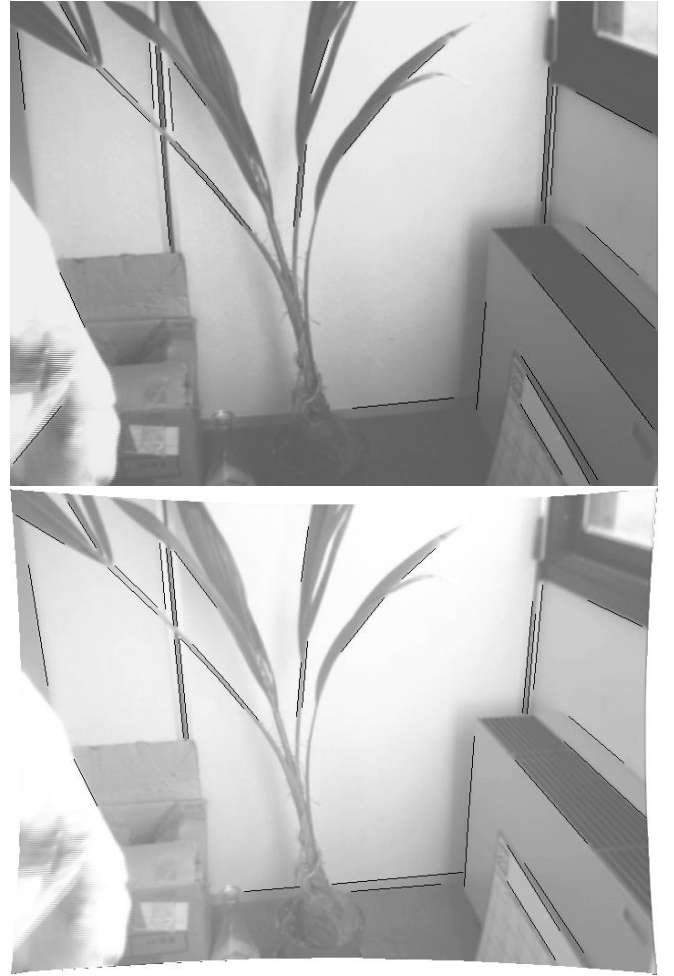
Fig. 5 A distorted image with the detected segments (left) and the same image at the end of the distortion calibration with segments extracted from undistorted edges (right): some outliers (wrong segments on the plant) were removed and longer segments are detected. This image represents the worst case, where some curves may be mistaken for lines.
