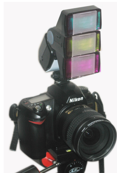
Figure 9. An hypothetical multi-flash system. The flash works in conjunction with the camera continuous shooting mode to capture three images, each with different added illumination.
