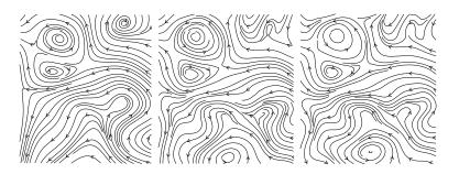
Figure 4: Motion field estimated on the OPA sequence, from the coarsest to the finest (full) resolution.
