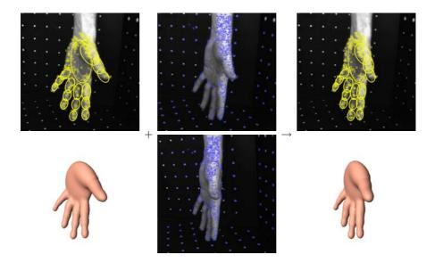
**Fig. 1.** This figure illustrates the alignment method described in this paper. *Left:* The articulated model (texture and surface) shown in its previously estimated pose, *Middle:* a set of 3-D data points obtained by stereo, and *Right:* the result of aligning the data (middle) with the model (left).
