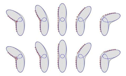
**Fig. 2.** The sliding of the texture onto a bending surface is controlled by the parameter a. For a = 2 (top) the texture nicely compresses and streches when the surface bends. For a = 10 (bottom) the texture is rigidly attached to the nearest rigid part.
