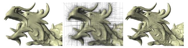
Figure 1: Left: simplified mesh of 15K triangles. Middle: an octree is built around this mesh to adaptively sample and store the normal field of the high resolution version of the mesh. Right: the simplified mesh is normal mapped via a special GPU traversal of the octree cells encoded in a 2D texture. The operation does not requires 2D parametrization of the mesh.
