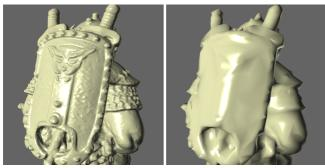
(a) Original (1.7M tri.) and simplified (5k tri.) meshes
