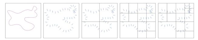
Figure 7: A 2D example of partitioning (i.e. quadtree instead of octree) according to the height map criterion  $\kappa$ . From left to right: the original shape, the corresponding point cloud with normals and successive refinement steps; each cell  $C_i$  whose associated point cloud  $P_i$  does not satisfy  $\kappa$  is subdivided.
