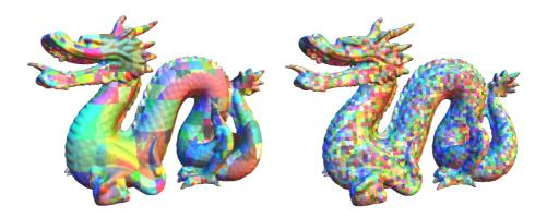
Figure 8: Partitioning criteria. Left: the piecewise mesh generated with a partitioning step only based on the  $\kappa$  criterion. Right: here, we have also included a maximum number of points by cell criterion.
