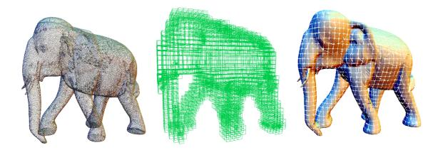
Figure 3: Reconstruction in each cell. Left: the initial point-based surface. Center: the cells of the space partition (in our case, the leaves of an octree). Right: a piecewise mesh independently reconstructed in each cell.
