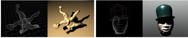
Figure 14: Surfel Stripping enables direct use of PBS in standard polygonal rendering engines. Here, two examples of antialiased Phong shading with shadow maps.
