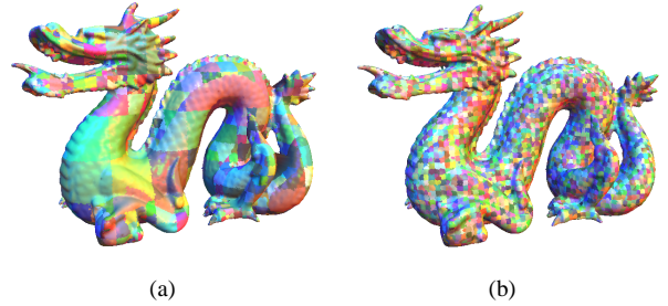
Figure 7: Partitioning criteria. (a) The piecewise mesh generated with a partitioning step only based on the \kappa criterion. (b) Here, we have also included a maximum number of points by cell criterion.
