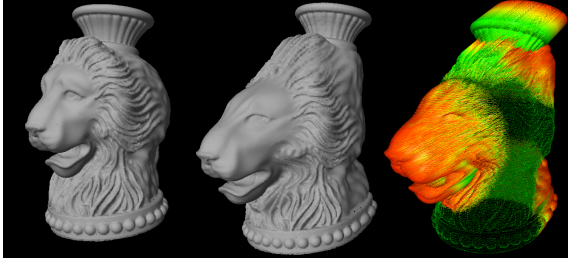
Figure 4: Left: Initial in-core geometry obtained by VS-Tree clustering. Middle: Deformed in-core geometry after an interactive FFD session. Right: Discrete displacement field generated by linking the initial (green extremum) and the final (red extremum) position of each sample point. This displacement field performs a sampling of the continuous space deformation function at the scale at which it has been edited.
