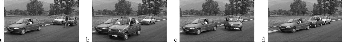
Fig. 12. Snapshots of a parallel parking: (a) localizing a free parking place, (b) selecting an appropriate start location, (c) performing a backward parking motion; (d) completing the parallel parking.
