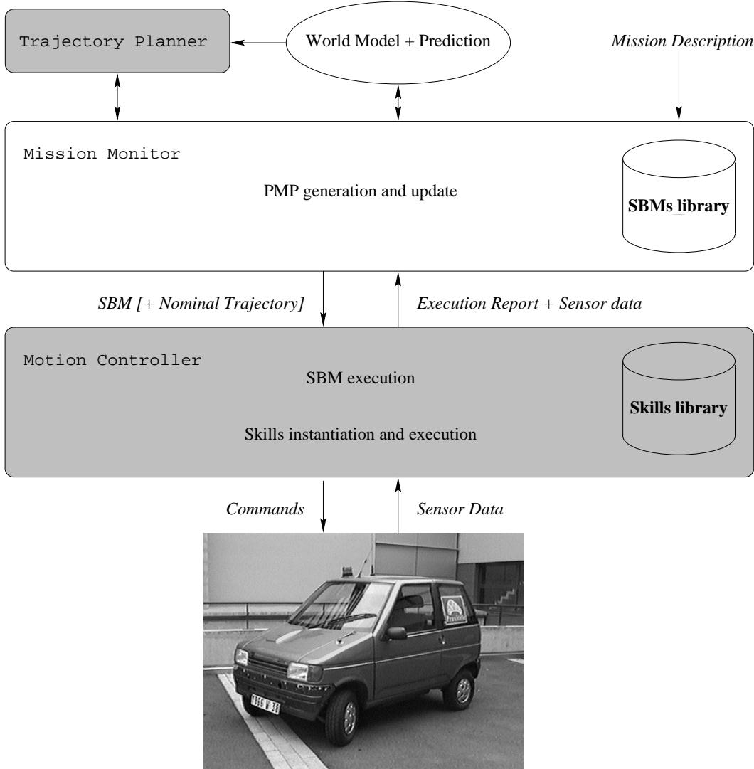
*Fig. 1.* The overall control architecture.
