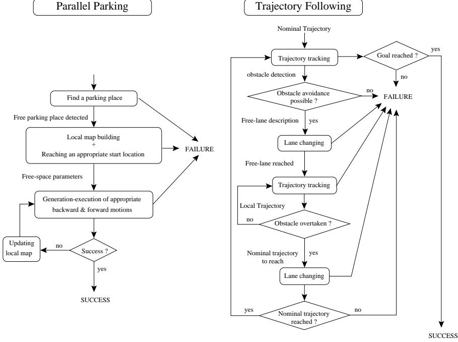
Fig. 6. The “parallel parking” and “trajectory following” SBMs.
