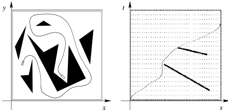
Fig. 3. (a) Path planning and (b) velocity planning.
