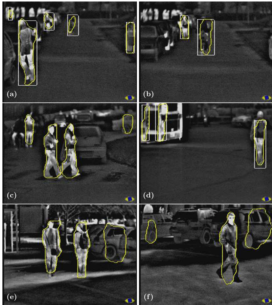
Fig. 5. Results: in (a) and (b), shape extraction of a close and distant pedestrian, respectively; the white snake represents the initial position, while the yellow one is the final configuration. In (c), a group of pedestrians is analyzed; in (d), a typical issue connected with a wrong initial snake disposition is shown: the head is outside the extracted shape because it was also outside the bounding box. In (e) and (f) some results in a difficult working condition are presented, i.e. during summer, when a lot of background objects appear bright, due to the high temperature.
