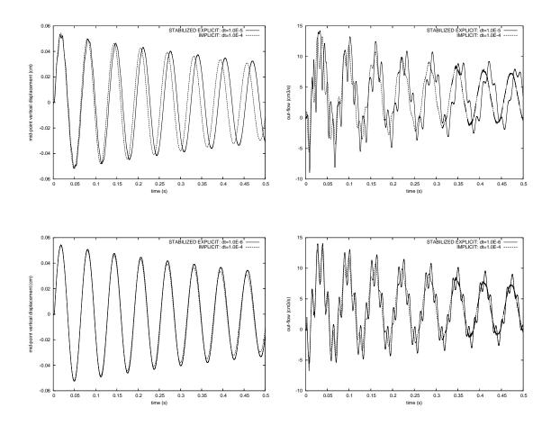
Figure 8: Interface mid-point y-displacement and out-flow, for  $\delta t = 10^{-5}$ ,  $10^{-6}$ , obtained with the stabilized explicit coupling (K = 0,  $\alpha = 1$ ,  $\gamma = 100$ ,  $\gamma_0 = 8.75 \times 10^{-4}$ ) and with the implicit coupling ( $\alpha = 1$ ,  $\gamma = 100$ ), for  $\delta t = 10^{-4}$
