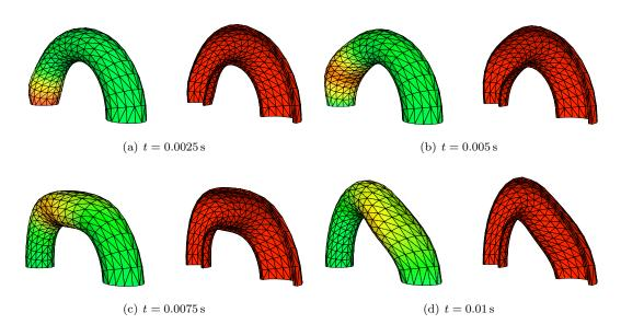
Figure 12: Curved vessel: snapshots of the pressure and solid deformation (exaggerated) at four time instants
