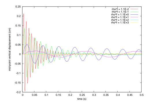
Figure 6: Stabilized explicit coupling  $(K = 0, \alpha = 1, \gamma = 100, \gamma_0 = 8.75 \times 10^{-4})$ : Interface mid-point *y*-displacement for different values of the fluid-solid density ratio  $\rho^{\rm f}/\rho^{\rm s}$
