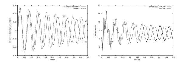
Figure 7: Interface mid-point y-displacement and out-flow: comparison of stabilized explicit coupling (K = 0,  $\alpha = 1$ ,  $\gamma = 100$ ,  $\gamma_0 = 8.75 \times 10^{-4}$ ) and implicit coupling ( $\alpha = 1$ ,  $\gamma = 100$ )
