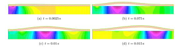
Figure 4: Stabilized explicit coupling (K = 0,  $\alpha = 1$ ,  $\gamma = 100$ ,  $\gamma_0 = 8.75 \times 10^{-4}$ ): snapshots of the pressure and solid deformation (exaggerated) at four time instants.
