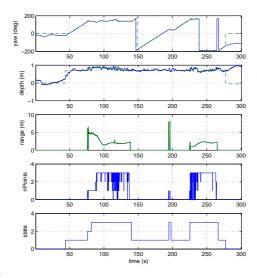
Fig. 4. AUV pose and SSL detection properties during a typical target identification and homing experiment. Here the AUV was required to identify the target and maintain a stand-off distance (range) of 2m.
