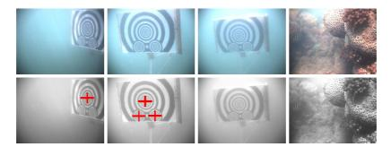
**Fig. 1.** SSL detection in marine environment. Upper row: original images, lower row: detection. From left to right: robustness to perspective and lighting discontinuity, minimum required contrast, insufficient contrast, absence of false positives in a natural environment.
