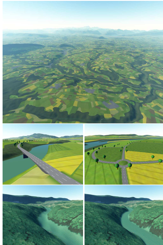
Figure 14: Results. Top: large scale view. Middle: procedural bridges and roundabouts. Bottom: with our footprints (right) rivers are flat even if the raw elevation data lacks precision – which is often the case (left). NB: here the texture is a satellite photograph.
