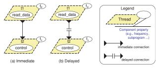
Fig. 1. AADL inter-thread data communication.
