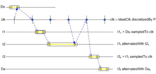
Figure 22. CCSL constraints, mixed case.
