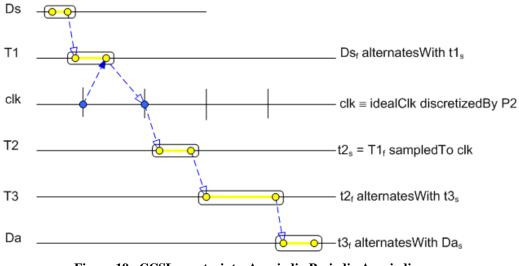
Figure 19. CCSL constraints, Aperiodic-Periodic-Aperiodic case.
