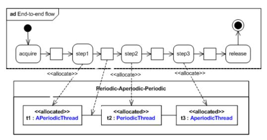
Figure 18. MARTE model, Aperiodic-Periodic-Aperiodic case.
