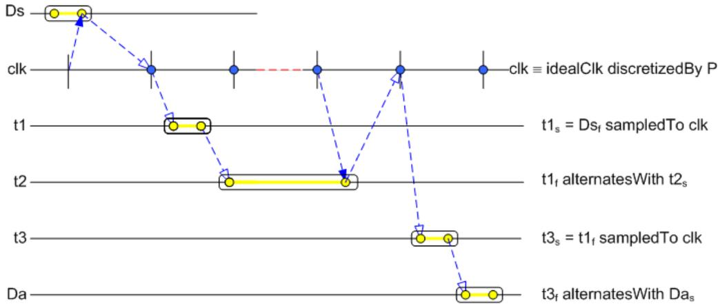
Figure 22. CCSL constraints, mixed case.
