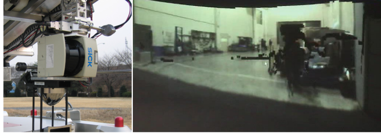
Fig. 9. Proposed sensor unit and obtained 3-dimensional information
