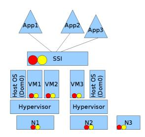
Figure 7: SSI Upon Type-I Virtualization
