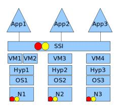
Figure 9: SSI Upon Type-II Virtualization
