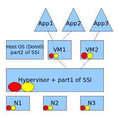
Figure 6: Type-I Virtualization Upon SSI
