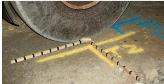
**Fig. 7.** Example positioning measurement from a test run, where the orthogonal lines marked ‘T2’ show the desired pose of the wheel’s outer edge.
