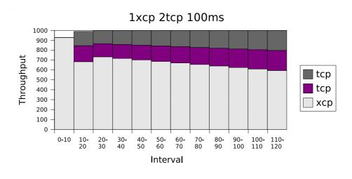
Figure 2: One XCP flow dealing with two concurrent TCP flows
