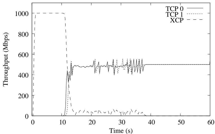
Figure 1: XCP flow dealing with TCP concurrent flows
