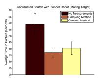
**Fig. 4.** Coordinated search results on a Pioneer robot comparing two methods for incorporating range measurements. Graphs show average capture times for a single searcher finding a stationary target (left) and a moving target (right). Error bars are one SEM, and averages are over 24 trials. Graphs are zoomed in for comparison.
