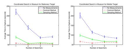
**Fig. 2.** Simulated coordinated search results in a museum comparing two methods for incorporating range measurements. Graphs show average capture times versus number of searchers for a stationary target (left) and a moving target (right). Error bars are one SEM, and averages are over 200 trials. Graphs are zoomed in for comparison.
