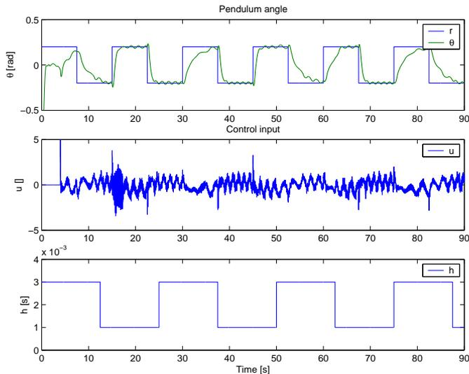
Fig. 13. Experimental motion of the T pendulum under a square sampling period
