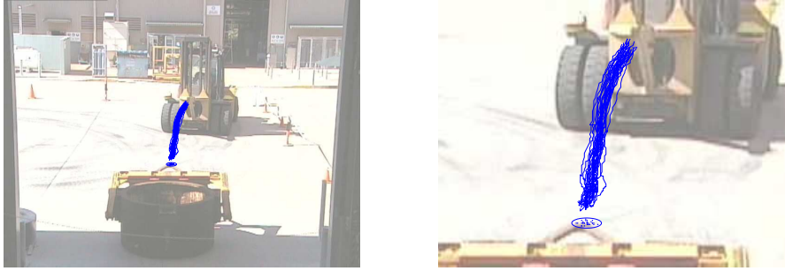
Fig. 9. Pickup approach trajectories, superimposition of 29 pickups. Dots and ellipse around the crucible handle show the variability of the crucible location across this set of manoeuvres. The left figure shows an overview of the stage, right figure shows a close-up on the paths themselves. For reference, the handle width is about 2 m and the pickup hole approximately 20 cm across.
