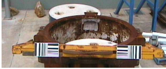
Fig. 6. Fiducial and their placement on the crucible
