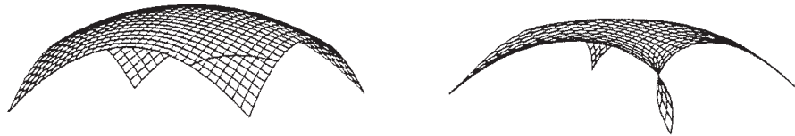
Fig. 6. Bicubic surface patch with line of vanishing Gaussian curvature (left). Orthotomic analysis (right).
