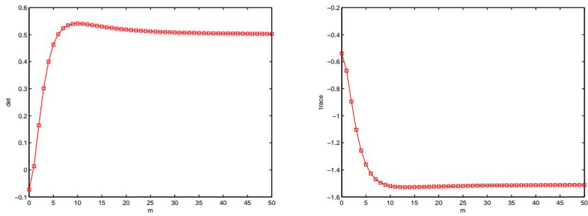
Figure 5: Plots of the determinant (left) and trace (right) of the matrix giving stability conditions (26) for the bumps pair ( $r_e = 3, r_i = 4$ ). These bumps are not stable since the determinant is negative for  $m = 0$ .
