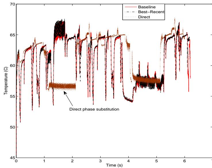
Figure 7: Temperature at the center of the instruction cache for *gcc* with baseline DTS compared to direct phase substitution and best-recent phase substitution. Thermal throttling is disabled. The number of intervals simulated in detail are 12 and 118 with direct and best-recent phase substitution respectively.
