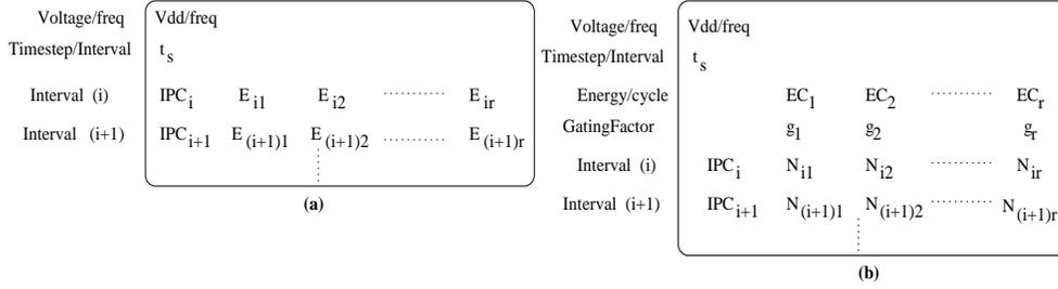
Figure 3: Partial trace contents. (a) Accurate format which consists in storing the energy consumed by each unit over a period of  $t_s$  cycles. (b) A simpler more compact format in which resource utilization counts are stored along with the baseline per-resource energy values.
