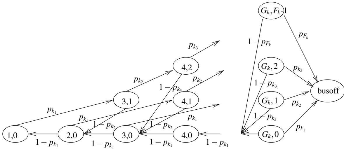
Fig. 8. Markov chain for the analysis of the proposed fault-confinement mechanisms where  $\beta = 1$ ,  $\alpha_1 = 2$  and  $\alpha_2 = 1$ . The value of  $G_k$  is  $\sum_{j=1, \dots, F_k-1} \alpha_j$ .
