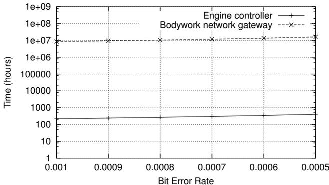
Fig. 7. Average hitting time of the bus-off state for the engine controller and the bodywork network gateway with the BER varying from 0.0005 to 0.001 and  $F_k = 31$  for the bodywork network gateway and  $F_k = 18$  for the engine controller (smallest value of  $F_k$  for the 6 nodes of the application).
