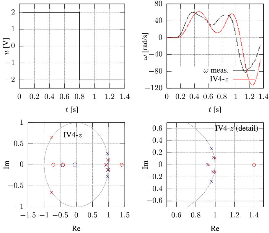
**Figure 9.** (cf. Example 6.6) Results obtained from measurements by invoking the standard instrumental variable method (IV4) implemented in MATLAB with  $\tilde{m} = m$ ,  $T_a = 10\text{ms}$ .
