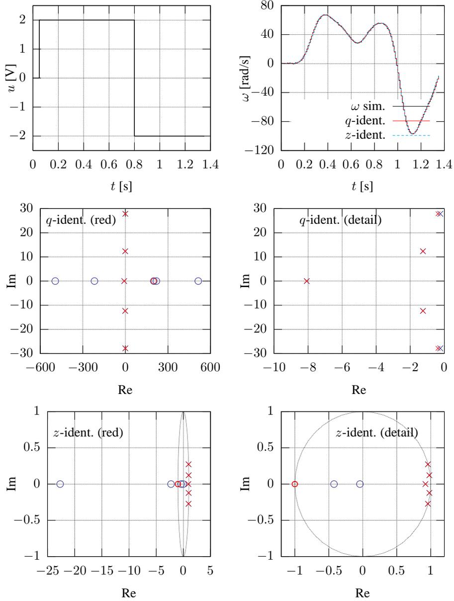
**Figure 4.** (cf. Example 6.2) Simulation results,  $\tilde{m} = 0$ ,  $T_a = 10\text{ms}$ . The usefulness of the idea of approximating the numerator in the sense of Sections 3 and 4 is verified, see also Figure 5 for the Bode plots.
