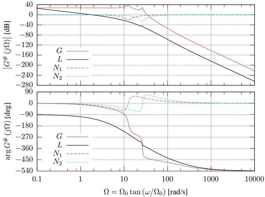
**Figure 10.** Control application: Bode plots of the identification result  $G^\#(q)$  due to the measurements of the lab model (c.f. Figure 7), and the plots of the Notch filters  $N_1$ ,  $N_2$  and the open-loop transfer function  $L = RG$ .
