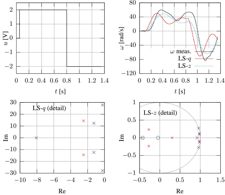
**Figure 8.** (cf. Example 6.4) Results obtained from measurements by invoking the standard least-squares (LS) method with  $\tilde{m} = m$ ,  $T_a = 10\text{ms}$ . The representations in terms of  $\lambda$  and  $\Lambda$  are entitled as “LS-z” and “LS-q” for short.
