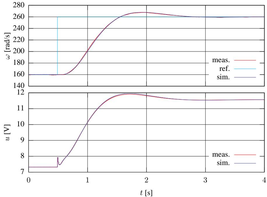
**Figure 11.** Control application: measurement and simulation results of the control system subject to a step change of the reference angular velocity.
