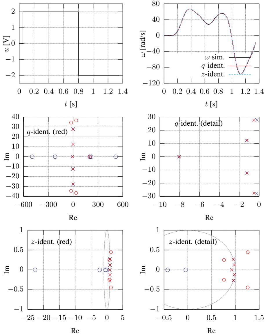
**Figure 2.** (cf. Example 6.1) Simulation results,  $\tilde{m} = m$ ,  $T_a = 10ms$ . Both  $z$ - and  $q$ -domain setting provide good results (regarding the system dynamics in the “interesting” frequency domain, see the system response and the Bode diagrams of Figure 3). However, the estimation of the zeros of both parameterizations is very inappropriate indeed.
