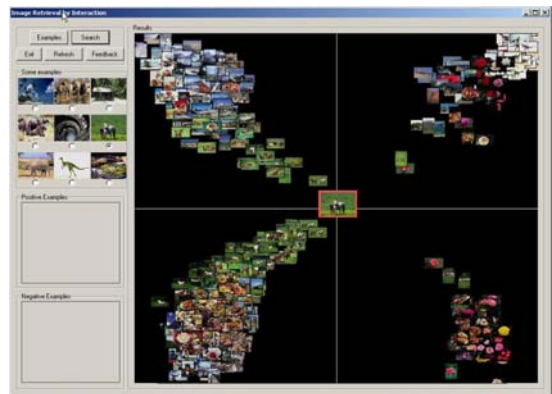
Figure 3. Results without relevance feedback, image query is center of the screen, image results are shown along to two axes: the vertical axis using the intersection histogram in RGB color space, the horizontal axis using the intersection histogram in HSV color space.
