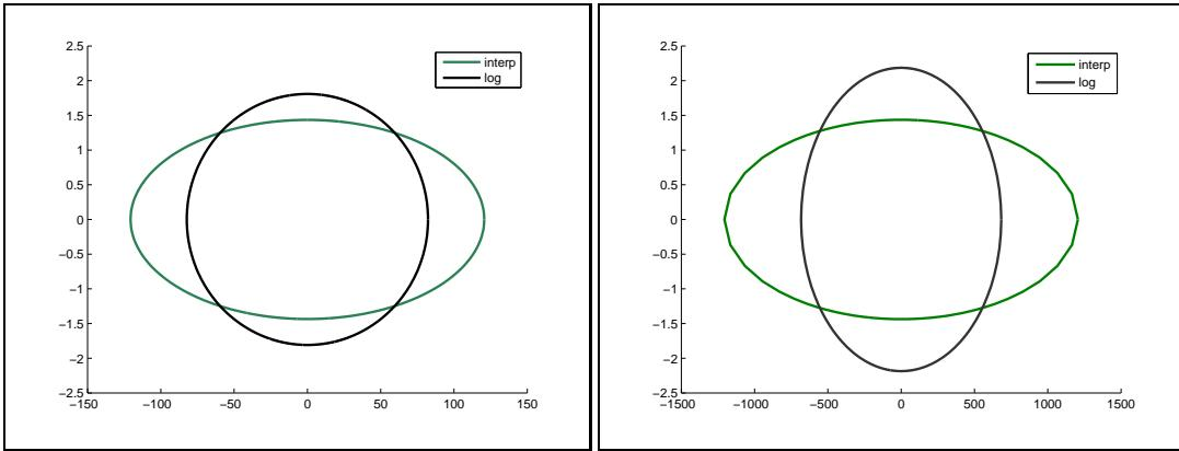
Figure 3: Comparison of the unit ball for the metric defined on the mesh of figure 1 with  $\alpha = 20^\circ$ . Left : Stretching ratio of 100; Right : Stretching ratio of 1000. Note that the units on the y-axis are scaled with a factor proportional to the stretching ratio in order to be able to visualize the unit balls
