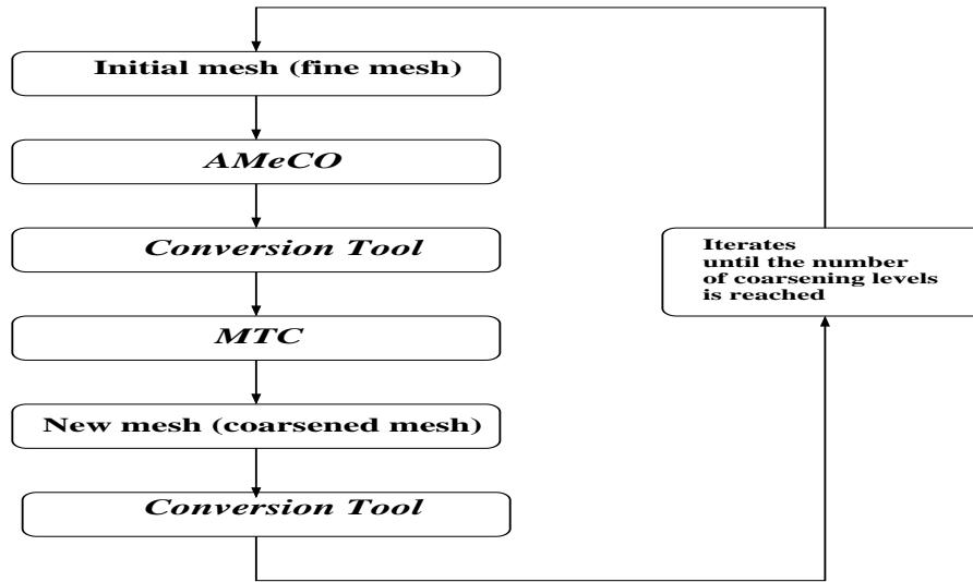
Figure 19: Coarsening process
