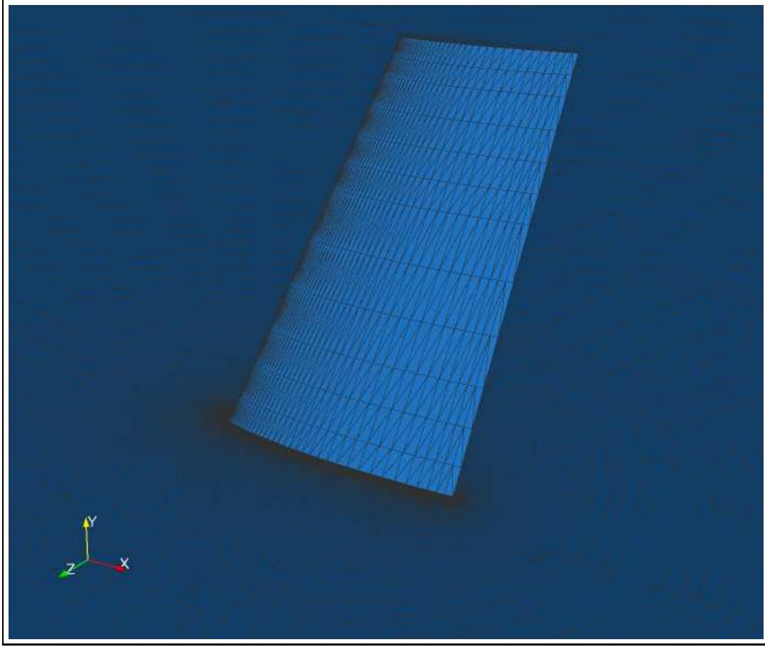
Figure 8: M6 wing : initial finest mesh
