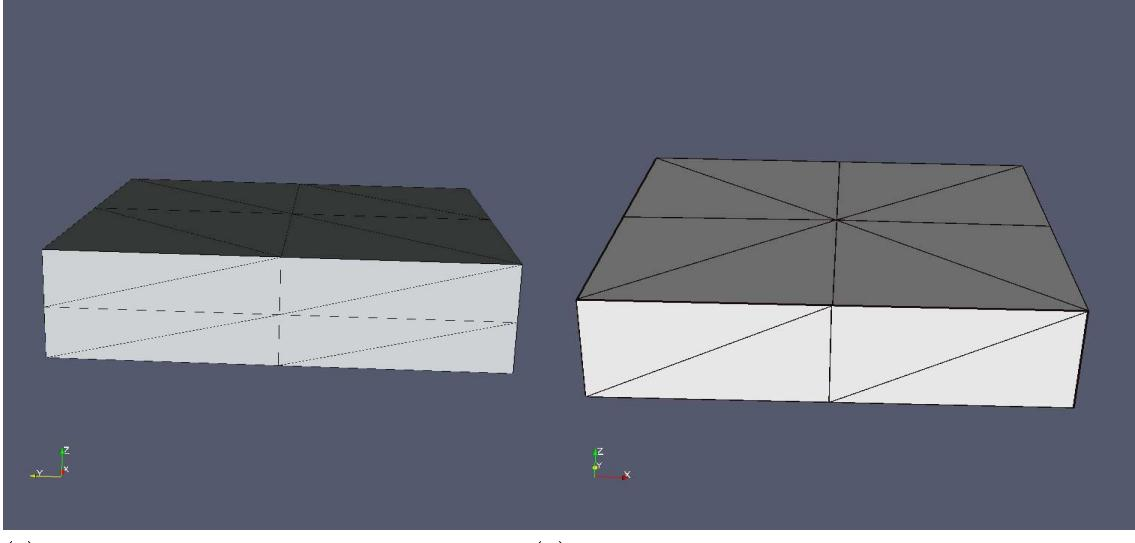
Figure 7: Semi-coarsening of a model boundary layer mesh. Note that the  $y$ -axis is scaled in order to be able to visualize the result.
