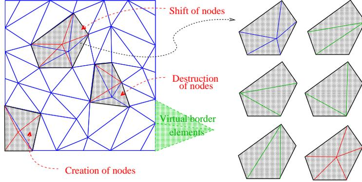
Figure 6: Local mesh optimization process in MTC
