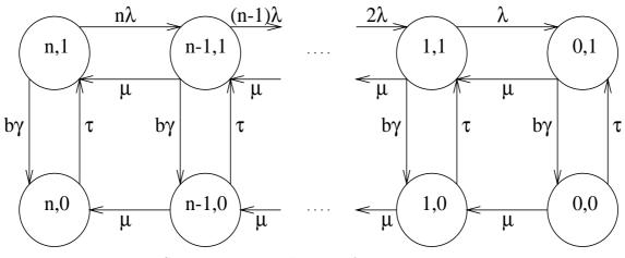
Figure 1: State-transition diagram for a *n*-processor system.
