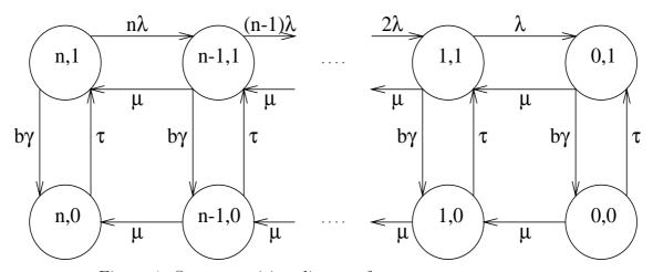
Figure 1: State-transition diagram for a *n*-processor system.
