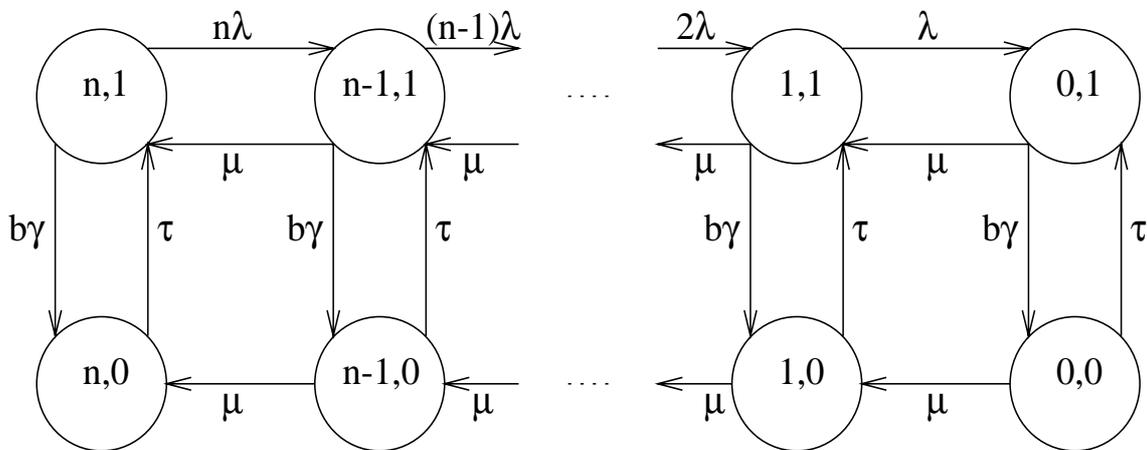
Figure 1: State-transition diagram for a  $n$ -processor system.
