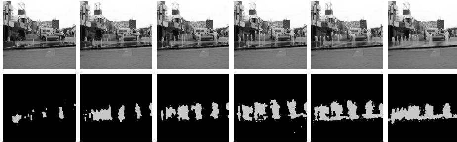
Figure 19: Segmentation of a sequence corresponding to a deformable motion texture of a fountain, using the graph-cut based method. The algorithm captures the varying shape of the segmented regions.
