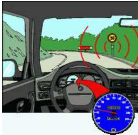
Figure 4.1: The active acceleration pedal interacts with the road a
