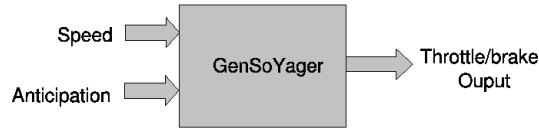
Figure 4.9: The throttle/brake subsystem scheme, anticipation added
