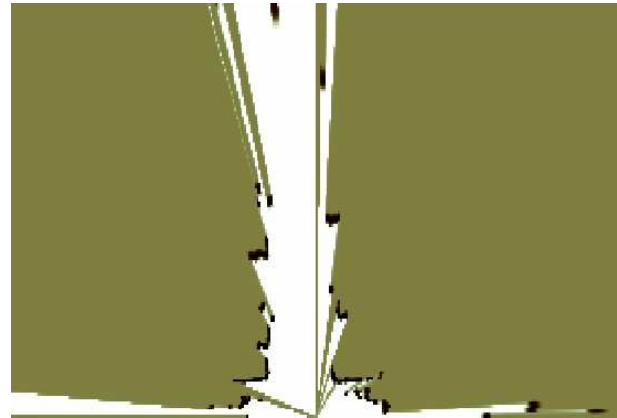
Fig. 6. Occupancy grid obtained from a laser range-finder.
