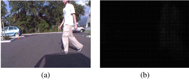
Fig. 3. Figure (a) is an image from a video sequence where the camera is translating and the pedestrian is moving in front of the robot. Figure (b) is the corresponding optical flow computed with [3]. Note the incorrect optical flow vectors on the ground plane.
