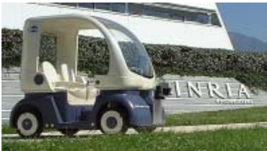
Fig. 1. The CyCab experimental vehicle. It is equipped with a Sick laser range finder.
