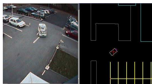
Fig. 15 The ParkView platform: left ) camera view of the Cycab experimental car moving in the parking lot of the laboratory; right ) the Cycab as detected on the tracking system.
